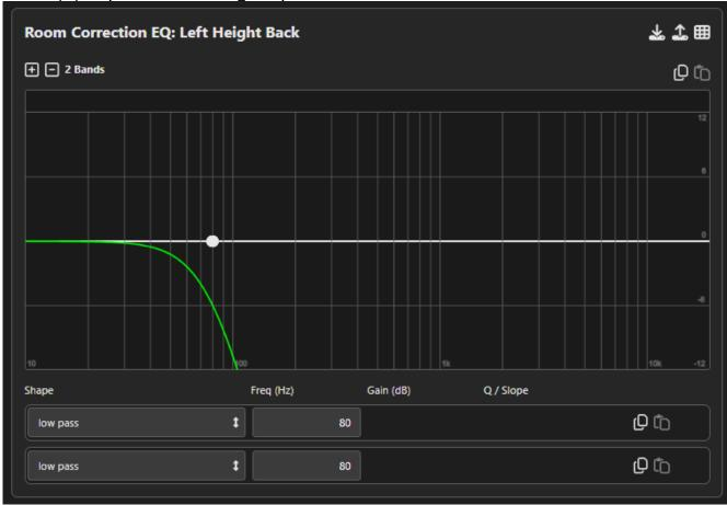
7. The outputs from the Height Low Pass speakers can then be connected to a sub-woofer. If the sub does not have Left and Right inputs then a passive summing network can be fitted inside and XLR connector to sum the left and right together.
